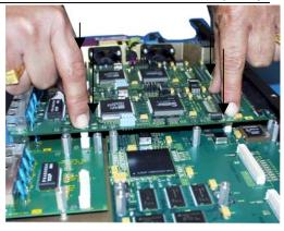
Figure 3.6.2f: Securely latching up 6KPM Cards into a Magnum 6K16-Series
